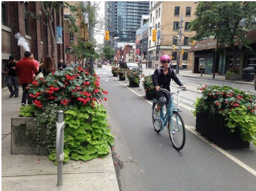
Figure 15. Image of a bike lane demonstrating planters as protective barriers
