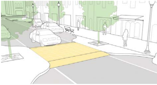
Drawing of a speed table in a complete street. With 500 feet between them, speed tables can limit the operating speed of automobiles in residential neighborhoods like that along S. Genesee Street to 25 to 30mph. Source: www.nacto.org .
